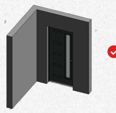
The model has parametric behavior. E.g: if a door is removed from the wall, the shape of the wall and its properties, like size and surface, will also change.
