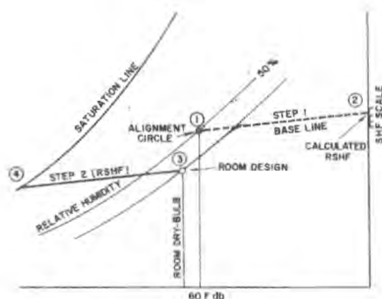
FIG. 35 — RSHF LINE PLOTTED ON SKELETON PSYCHROMETRIC CHART
